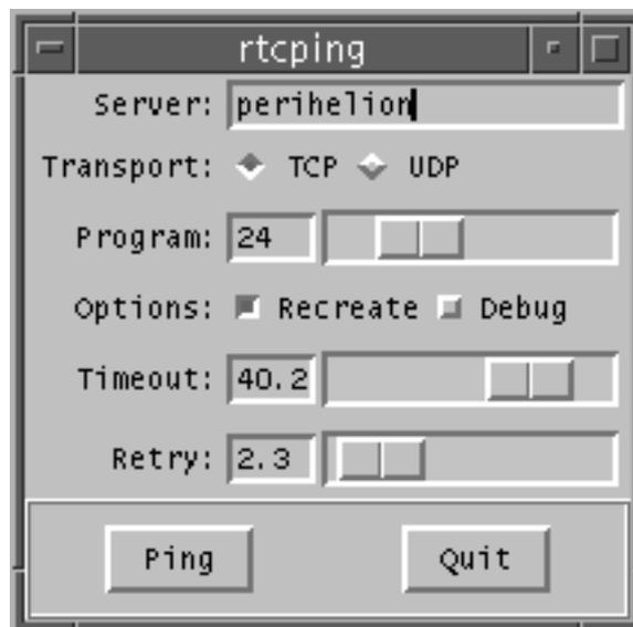
Operation is largely self-explanatory: the configuration of an RTC handle can be altered using the widgets at the top of the interface: a `ping` remote call is initiated by pressing the `Ping` button. If there is an error, a pop-up appears with the error string in it.
